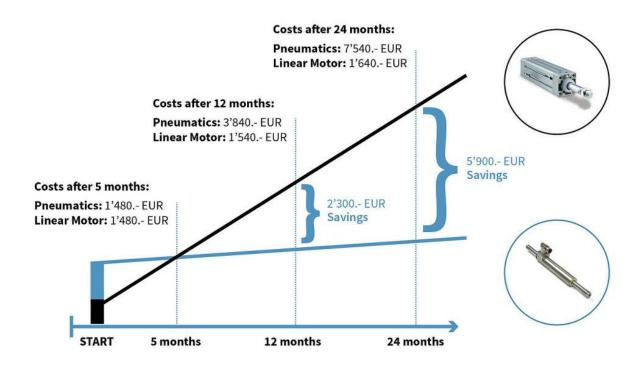
A linear drive, including all required components (cables, inverter, etc.), in contrast, does cost more than a pneumatic drive (including valves, tubing, etc.).
