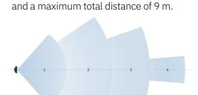
The aperture of each field is dynamically adjustable in  $10^{\circ}$  increments over a range of  $10^{\circ}$  to  $100^{\circ}$  (0-5 m) and over a range of  $10^{\circ}$  to  $40^{\circ}$  (5-9 m).
