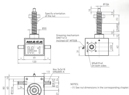
... Power required:  $P_{D}$  (kW) = 0.157x  $M_{D}$  (Nm).
